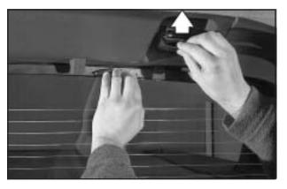
Push the rear glass flat against the window frame and push each latch lever up until it locks. You should hear a click when each latch lever locks correctly.
